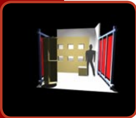
3-D CAD model used for early proposal. This helps avoid size and space problems later on.
